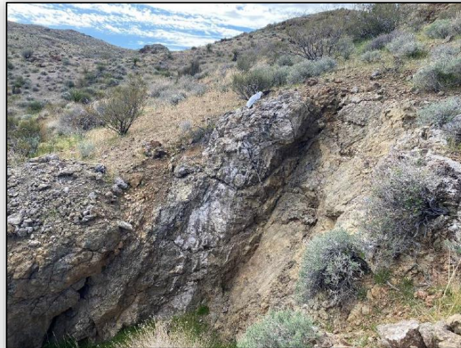
Middle Dixie prospect: Bladed quartz-calcite vein with quartz-rich bands– 1.0 m @ 3.27 gpt Au
