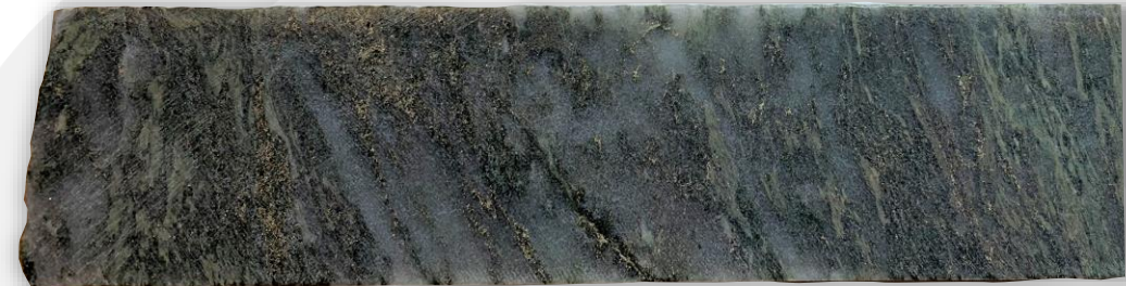
DD22SK004 – Silica flooding with pyrite-pyrrhotite replacement and vein fill.
