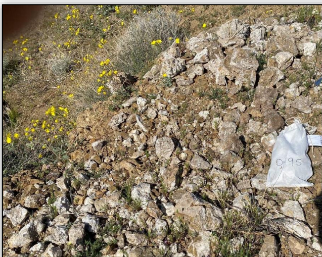
Cottonwood prospect: Massive calcite-quartz vein – 34.1 gpt Au
