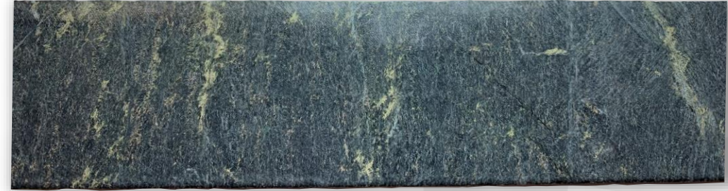
DD22SK002 – Abundant pyrite-chalcopyrite in sheared mafic volcanics.
