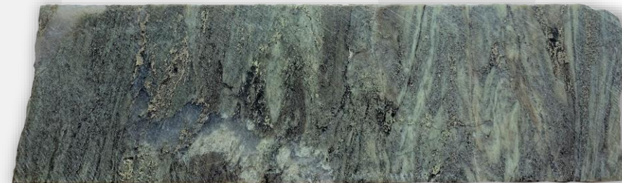
DD22SK006 – Abundant pyrite-pyrrhotite in silica-sericite-illite altered shear zone.
