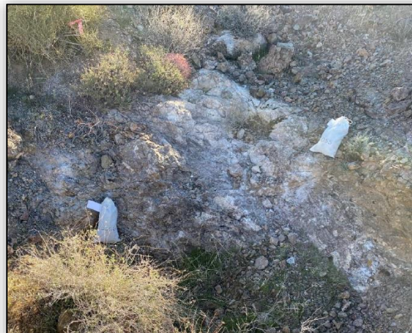
Golden Ram prospect: Chalcedony-calcite vein breccia – 1.4 m @ 4.09 gpt Au
